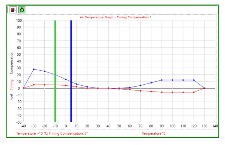
When air is cold it is denser and requires more fuel for the same AFR readings. When air gets hot you can lean out the fuel a bit on the blue line. The timing can also be advanced a bit for cold air and retarded for warm air. For Turbo engines hat air sometimes is cooled off by adding fuel to prevent melting the pistons. Notice the first and last digits are set to zero. This helps if the sensor breaks to disable compensation.
